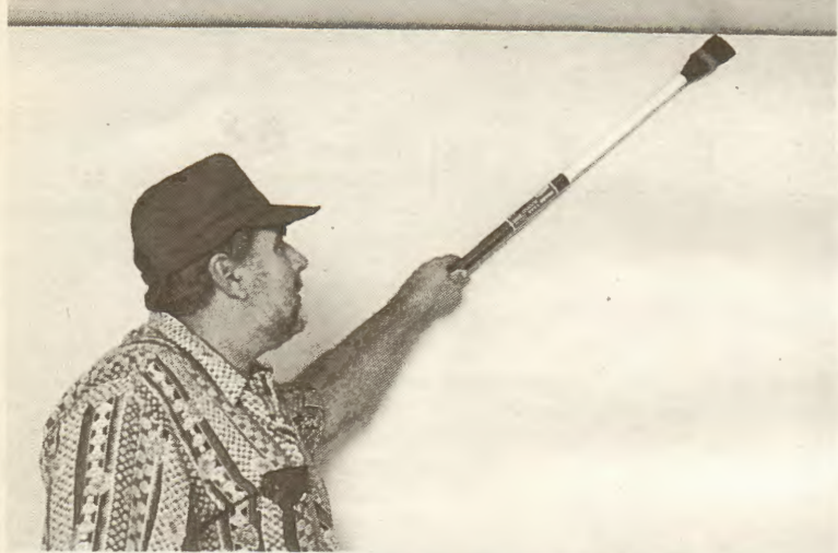
AB Richard Wheat demonstrates the versatility of his patented invention: a paint brush which can be screwed directly onto a pole.
