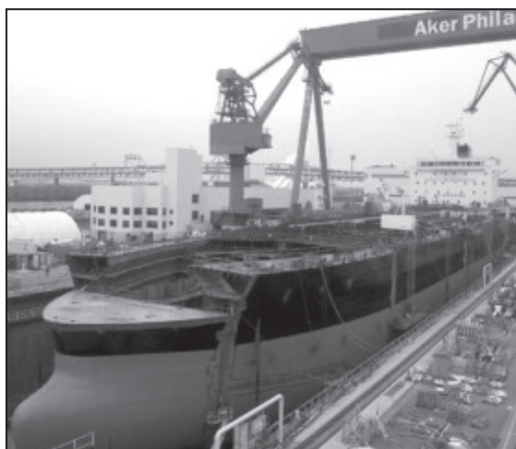
Tanker construction is ongoing at Aker Philadelphia Shipyard, where the fourth vessel in the Veteran Class series (above) now has its rudder and propeller attached, with the deckhouse also set in place.
