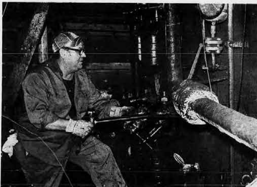
SIU veteran Charles Sharp, who sails as fireman, cleans off a burner rod in Bethflor's engine room.
