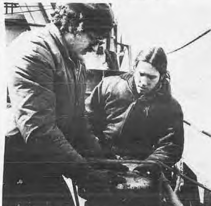
AB-Watchman Dick Lovaas, left, makes a turn for the better as he and OS John Watson oil the vent caps of the John T. Hutchinson's ballast tanks.
