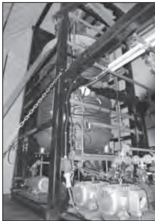
The ship is carrying two hydrolysis systems (including this one) designed to neutralize up to 25 metric tons of chemical warfare agents a day. (U.S. Army photo by Todd Lopez)
