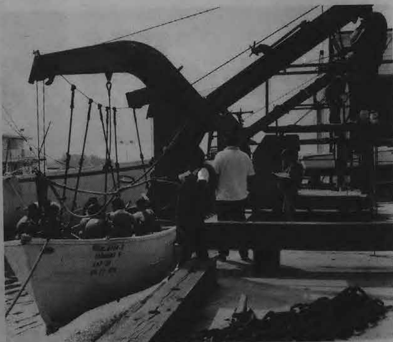
Davit launching is practiced by the Hawaiian crew members.
