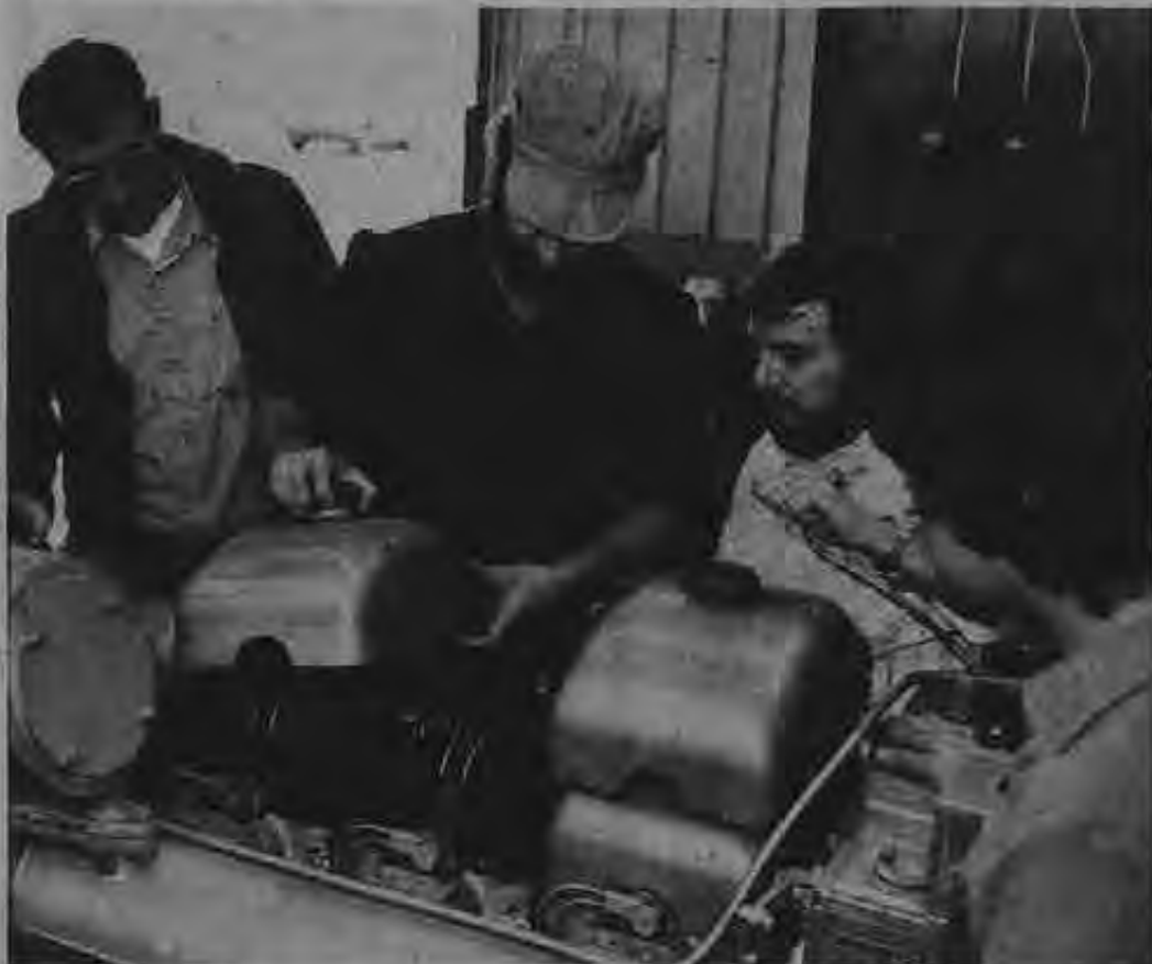
SHLSS Instructor David Grieg, left, works closely with his students in all phases of their diesel engine training. Here he watches as David Goulard, of Algonac, removes the cylinder valve cover from a GM 8-268 diesel engine. Seafarers James Luke, from Wilmington, and Stephen Duffy, Houston, stand by to assist.
