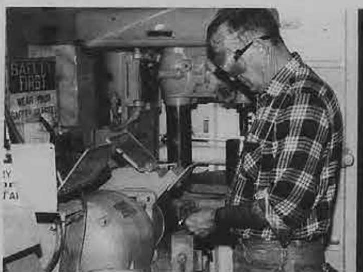
Burnishing a winch part on the wire wheel in the ship's machine shop is QMED Warren Redick.
