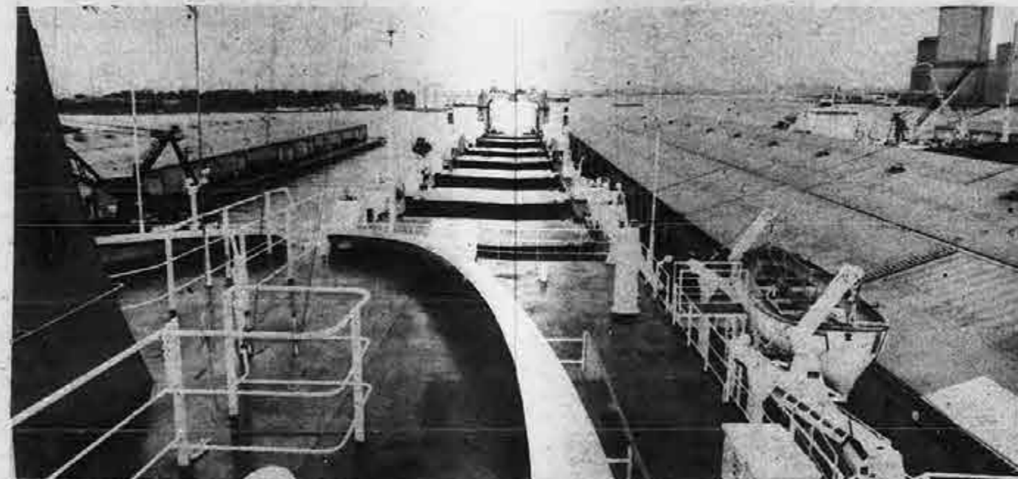
The view aft from the Stonewall Jackson's bridge, showing her barge holds and crane.
