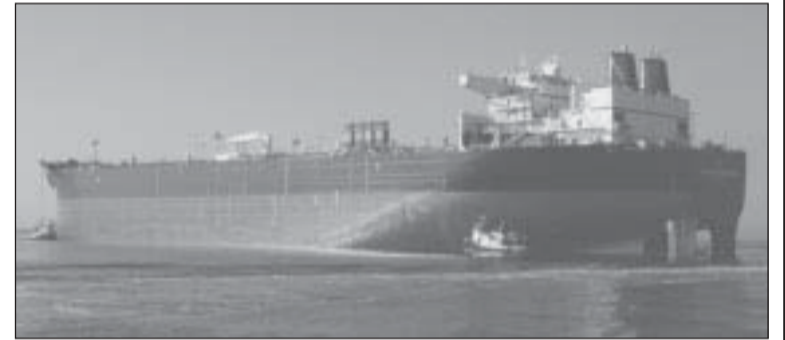
The Alaskan Frontier , scheduled for delivery in June, is one of four double-hull Alaska-class tankers being constructed on the West Coast. SIU-contracted Alaska Tanker Company will operate the new vessels.
