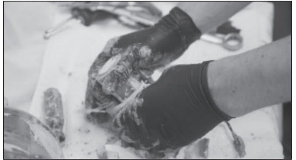
National Transportation Safety Board personnel (photo at left) monitor video from the remotely operated vehicle CURV-21 during the recovery of El Faro 's voyage data recorder capsule. In the photo above, an NTSB engineer removes material from the inner capsule assembly. (NTSB Courtesy Photos by James Anderson)
