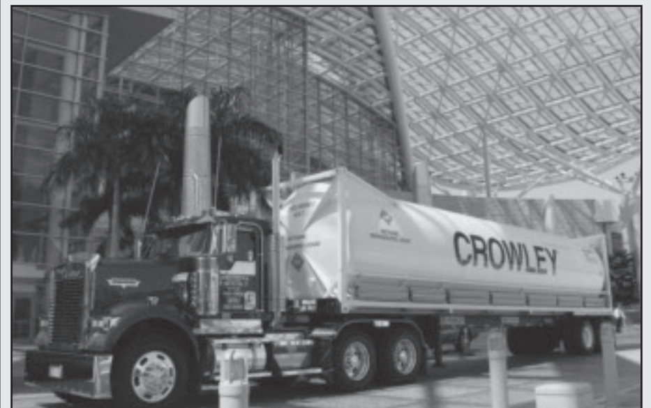
As part of Crowley's new contract, forty-foot ISO containers like the one shown above (authorized by the U.S. Department of Transportation) will transport 10,000 gallons of LNG from various U.S. mainland liquefaction facilities to the company's shipping terminal in Jacksonville, Fla. (Photo Courtesy of Crowley Maritime Corp)
