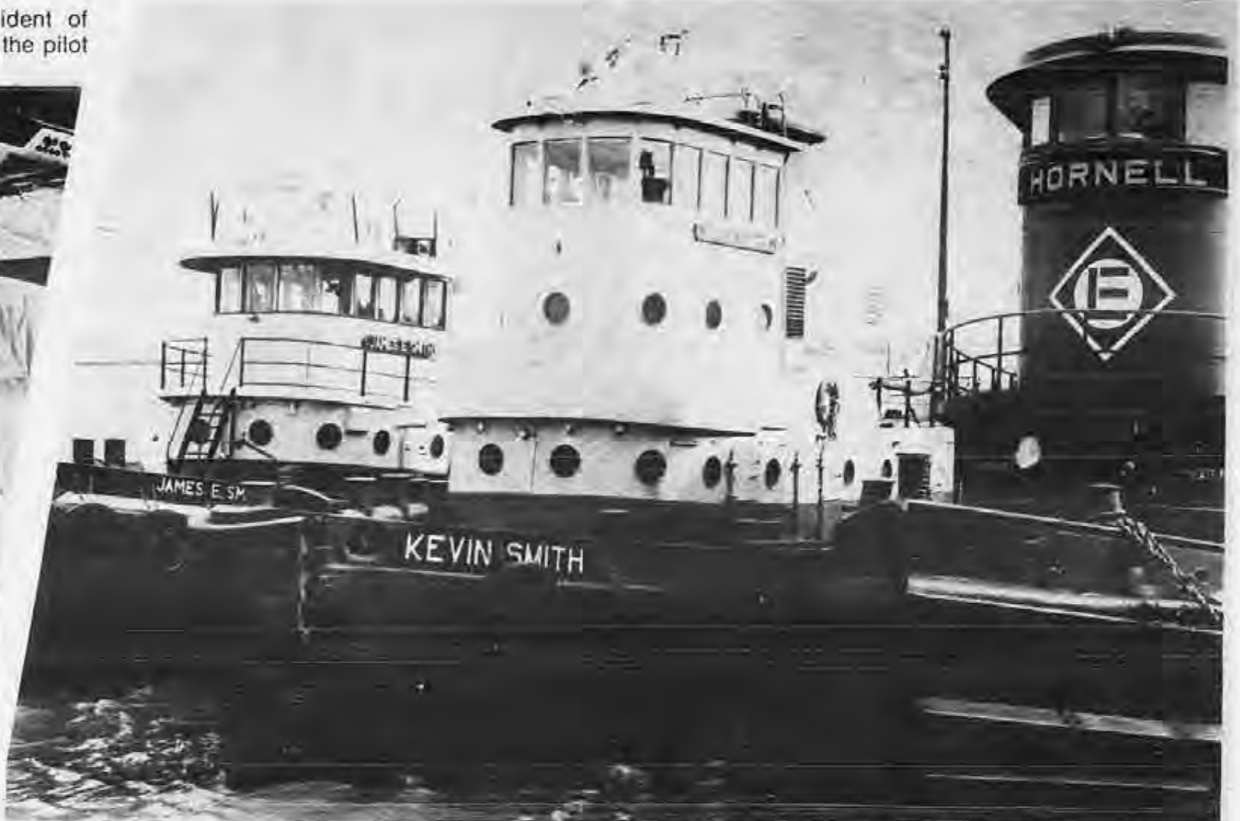
These three tugs show the changes that take place in Crescent's rebuilding program. The recently acquired Hornell , right, is a before picture of an old railroad tug. The Kevin Smith , center, has been repowered and remodeled but still has the old, high pilot house. The James E. Smith , left, with its lowered pilot house, is a completely re-built and up-to-date shipdocking tug.
