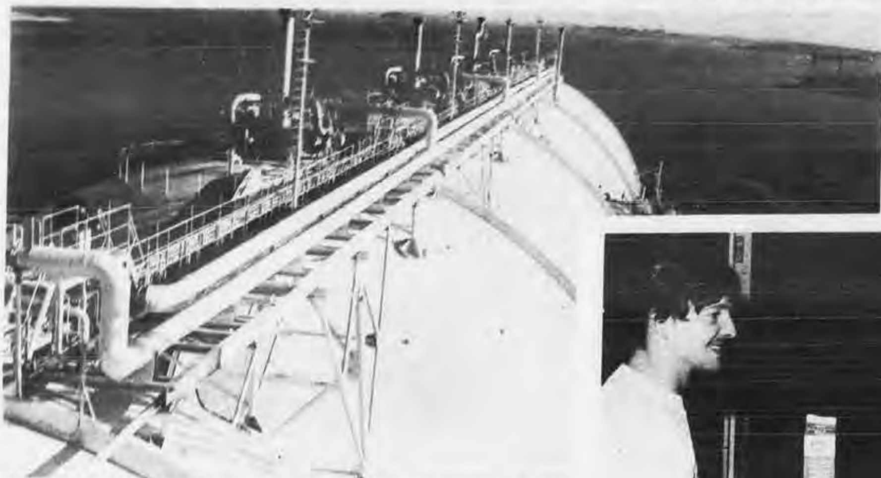
A view of the LNG Aries cargo tanks. The five tanks are designed to hold 125,000 cubic meters of liquified natural gas at a temperature of 265 degrees below zero F. Weighing 800 tons each, the tanks were constructed separately from the rest of the vessel and shipped by barge to the shipyard.
