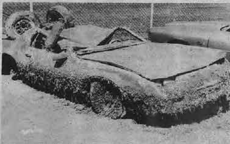
The small, striped mollusk is very adaptable, finding almost any surface acceptable for attachment. Shown here is the effect of zebra mussels on a car which was submerged upside down in Lake Erie for one year.
