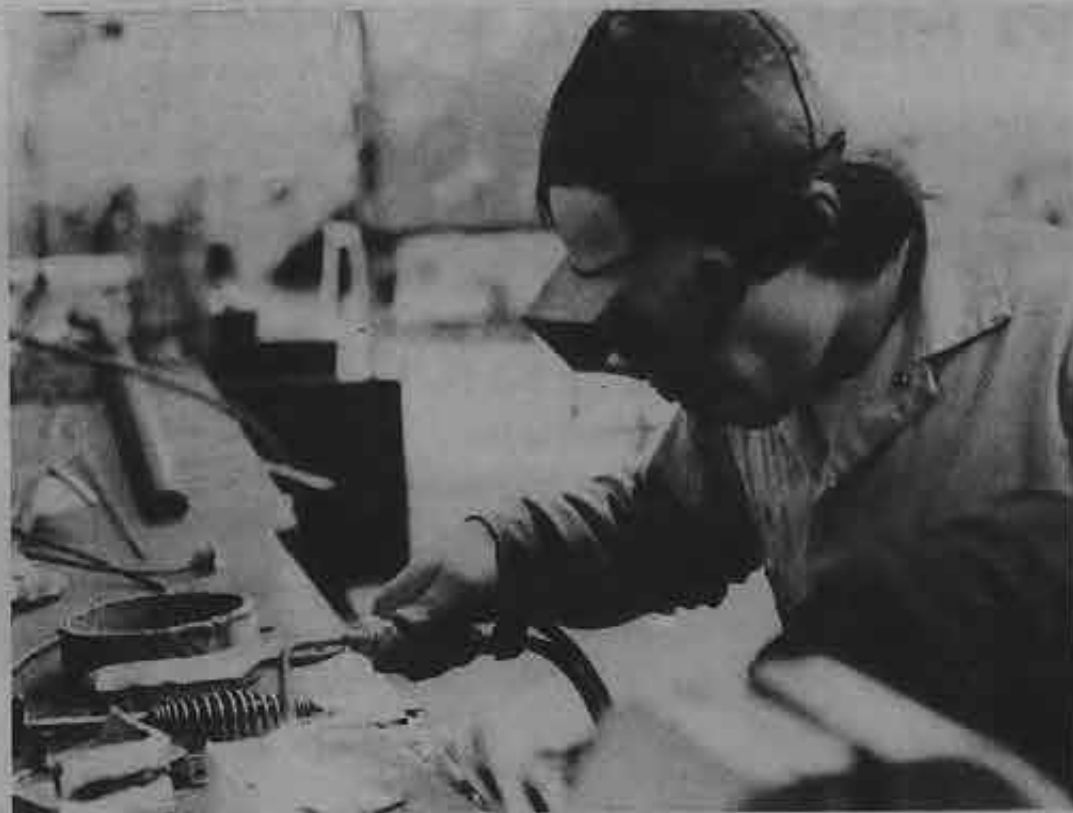
Dasril Panko brazes on a mild steel plate in the flat position.
