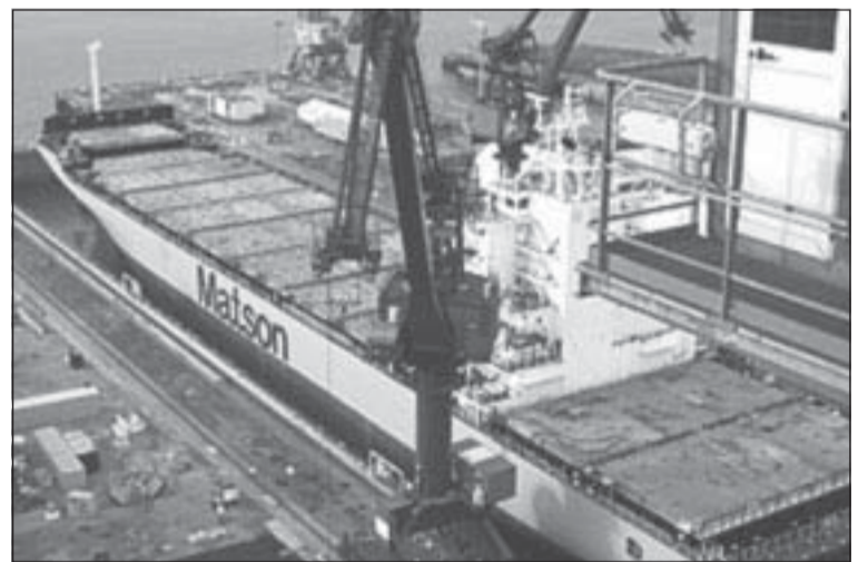
The third ship under construction at Kvaerner Philadelphia Shipyard, the Manulani , is a Philadelphia Class CV2600 containership under contract with Matson. Last month, the ship was floated in preparation for its final outfitting prior to delivery.
