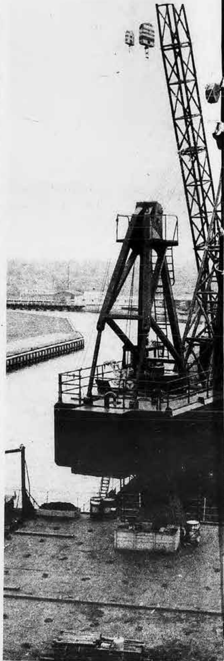
The Seatrain Florida 's twin 45-ton capacity deck cranes at the Port of Camden, N.J.
