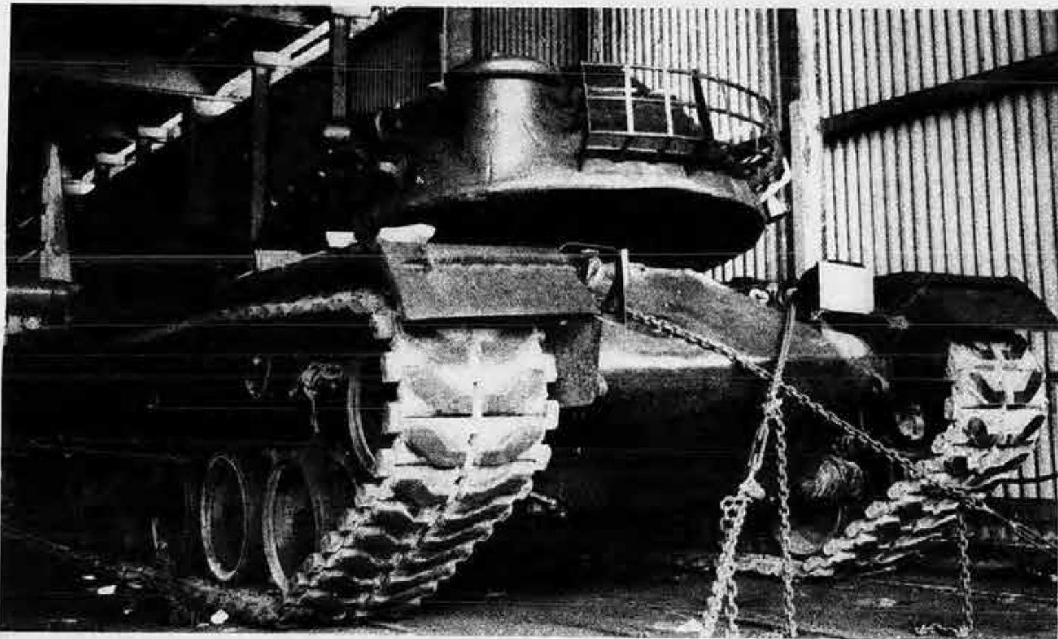
A sturdy U.S. Army tank, disarmed before loading in Saigon, is securely anchored to the converted deck of the Seatrain Florida .
