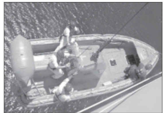
A few members of the deck department team haul the raft aboard the ship platform, which opens to the water level from the hull, midships.
