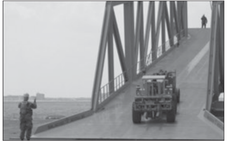
U.S. Navy Photo by Christine Albert Army vehicles roll off the SIU-crewed USNS Red Cloud onto a floating barge. The process is used when port facilities are not available.
