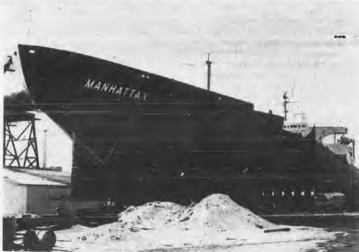
Looking at a front view of the supertanker TT Manhattan undergoing modifications to her icebreaking bow.
