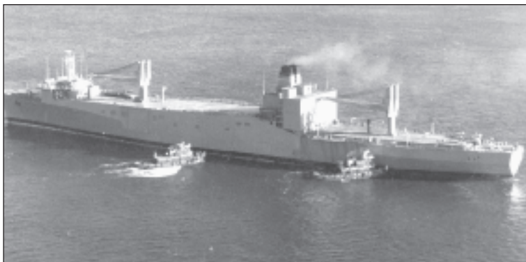
Like LMSRs, MSC's fast sealift ships (including the USNS Bellatrix , above) are roll-on/roll-off vessels equipped with on-board cranes and self-contained ramps.
