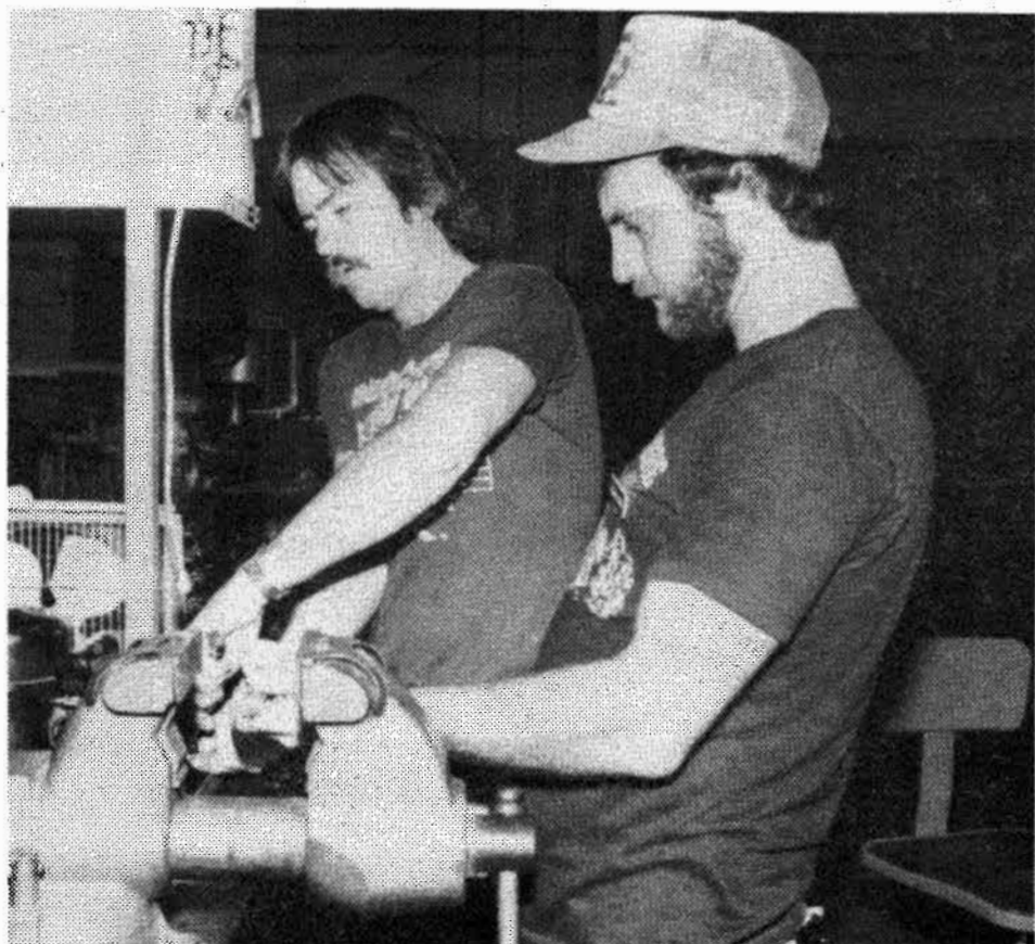
James McDaniel (l.) and William Lignos install a filter dryer and sight glass/moisture indicator into a liquid line.
