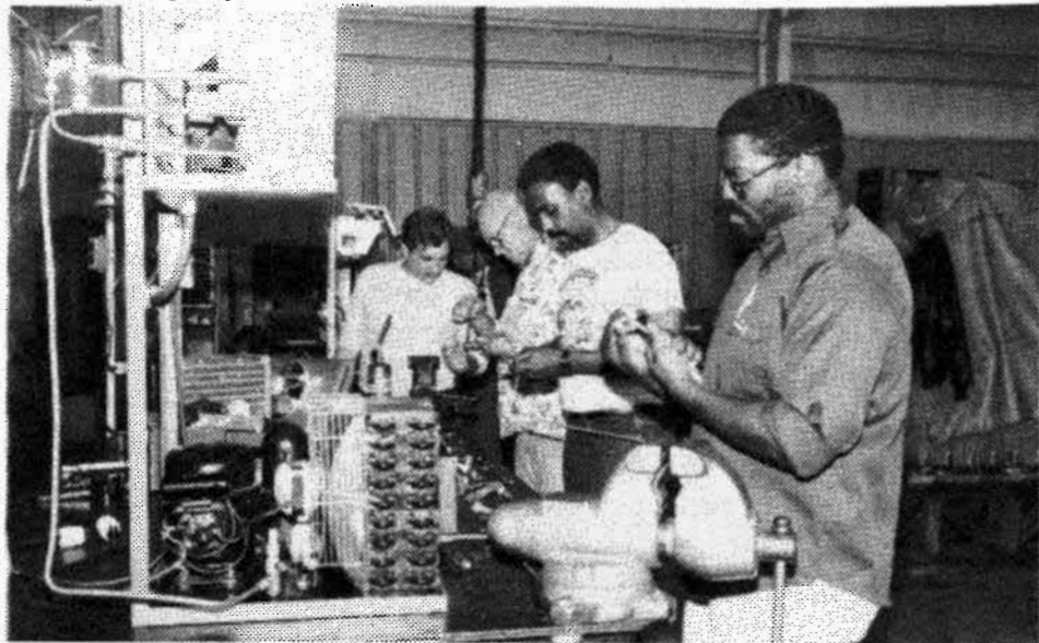
Tyler Womack (r.) prepares a joint for soldering. Left to r. Steve Walters and Edwin Harris inspect a soldered joint while Spurgeon Simpson cuts refrigeration tubing.
