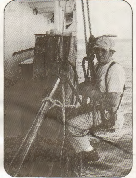
AB Russell Luther uses the bosun's chair to paint the hull of the Louis Hauge in Diego Garcia.
