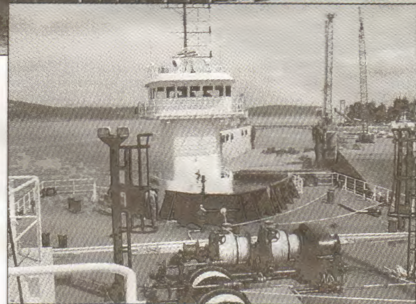
The tug and barge units of the ATB are connected in Ferndale, Wash. (top photo). The picture above shows, in greater detail, the tug in the notch of the barge.
