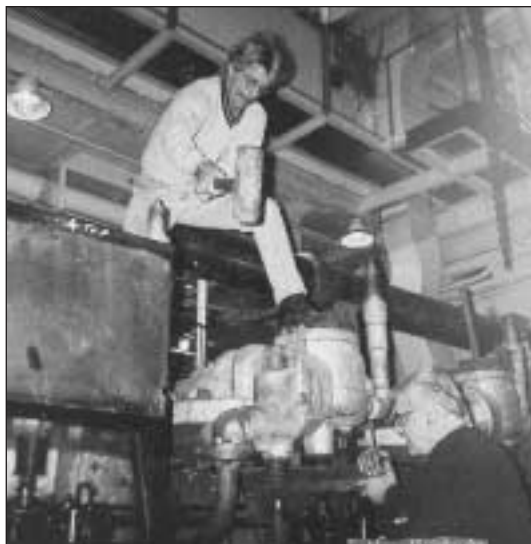
Oilers John Cull (left) and Andy Egressey prepare to pull the head on cylinder #2 of the main engine on the Southdown Challenger .
