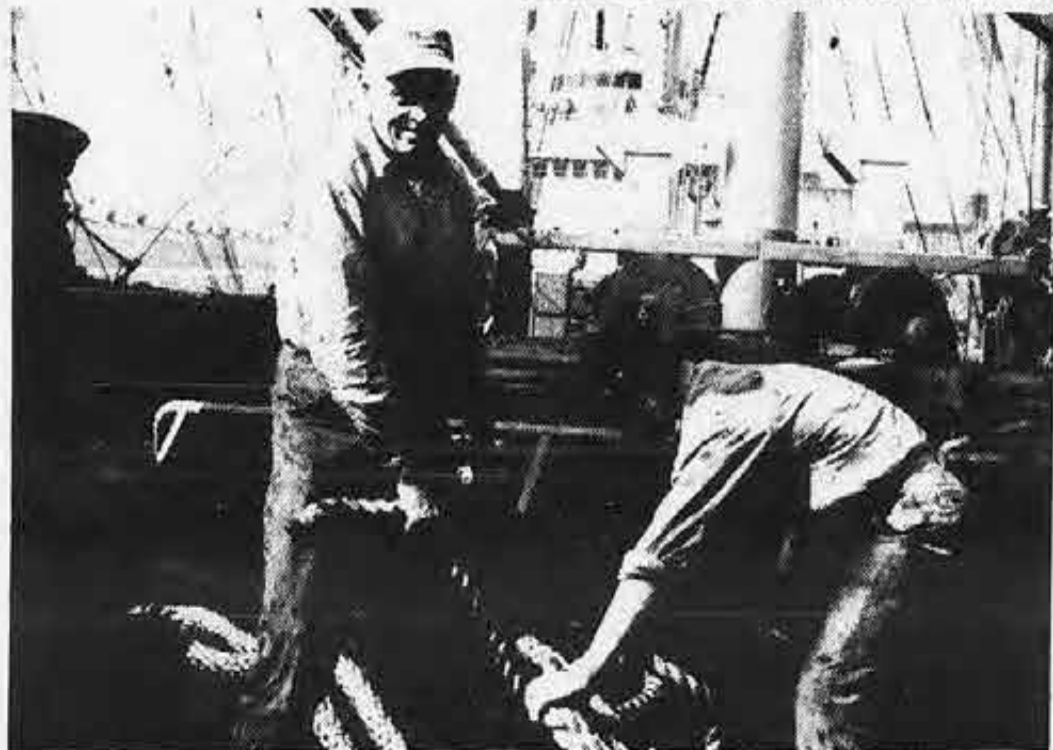
Seafarers Frank Liro and George Gallard bend to the task aboard the Robin Locksley while splicing the new improved mooring line. The new mooring line is made out of nylon, demonstrating yet another use that synthetic fibers are put to.
