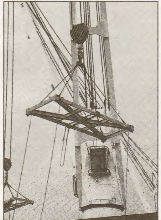
All cranes aboard the Pvt. Franklin J. Phillips were rigged with adjustable spreaders in preparation for cargo operations in Jacksonville.
