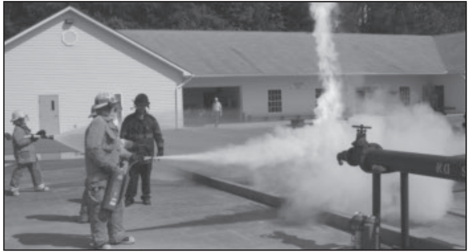
Special firefighting techniques must be used when dealing with an LNG fire, as demonstrated by these students.
