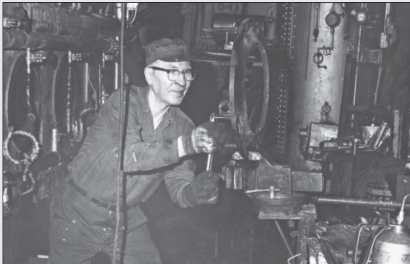
From the May 1976 Seafarers LOG : "Seafarer Francis Buttas stamps out flange on a damper that was stripped and needed a new thread. Buttas sails as fireman aboard the John T. Hutchinson ."
