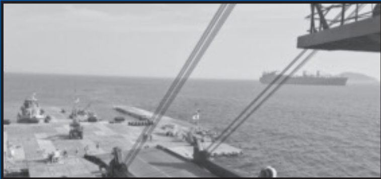
The stern ramp is lowered from the USNS Bobo . The ship is operated by SIU-contracted Maersk Line, Limited for the U.S. Military Sealift Command.
