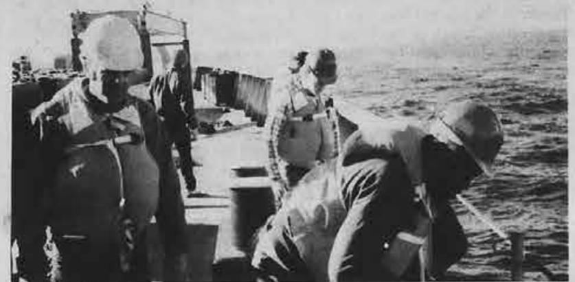
Bosun George Wilson directs the deck crew of the Denebola to seal the probe into the receiver during underway replenishment exercises between the Bay Tankers-operated vessel and the USNS Neosho.
