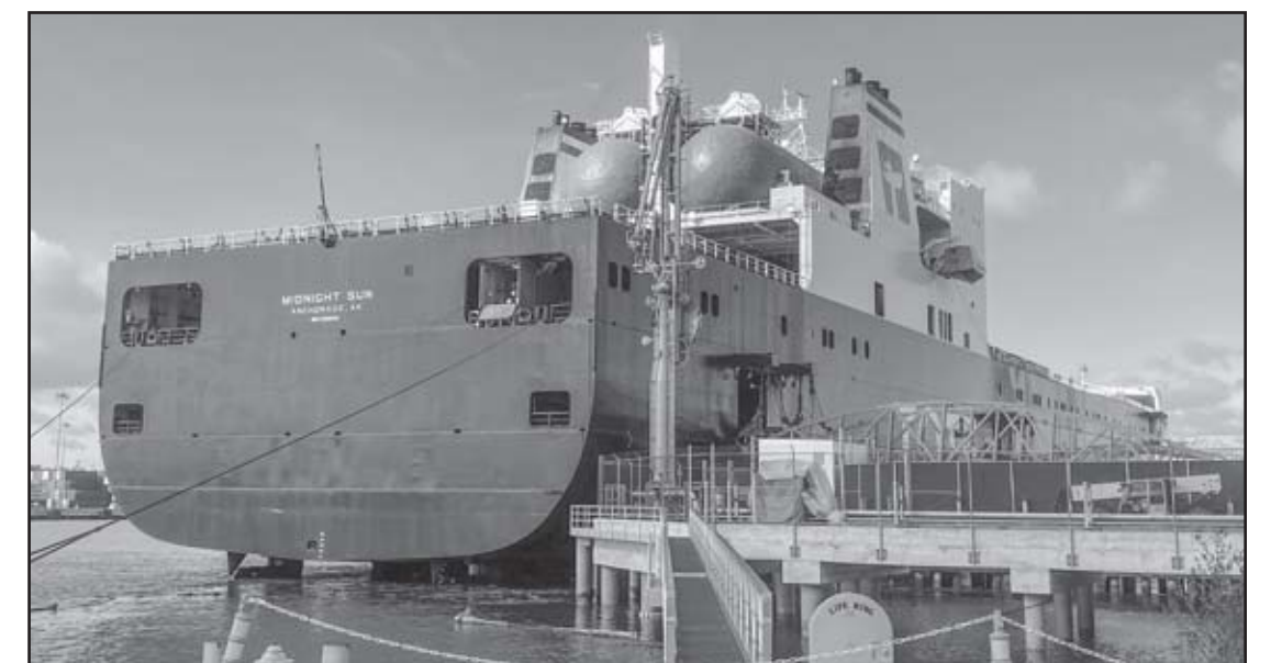
The project includes a new aft deck, two 1,100 cubic meter LNG tanks and supporting infrastructure, as pictured above. The Midnight Sun's conversion (photo below) to LNG fuel is slated for completion in 2022.
