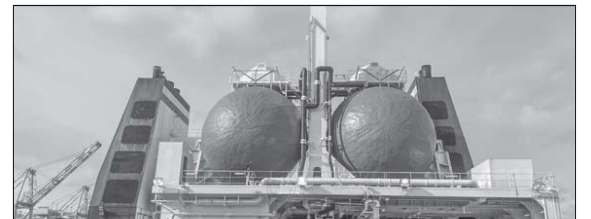
The project includes a new aft deck, two 1,100 cubic meter LNG tanks and supporting infrastructure, as pictured above. The Midnight Sun's conversion (photo below) to LNG fuel is slated for completion in 2022.
