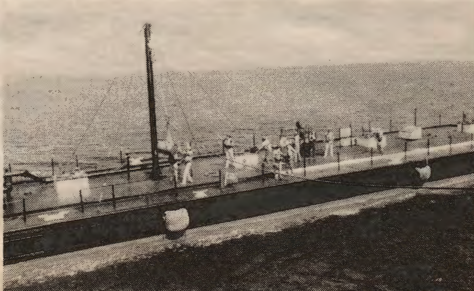
After the drum is received, it is disconnected from the chime hooks and is sent back to the delivery ship for an additional load.
