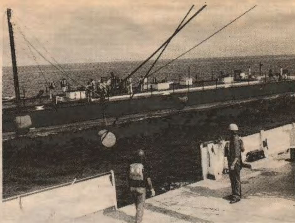
During an UNREP, a 55-gallon drum is hauled aboard the receiving vessel by means of the in-haul line, and is kept about 8 feet above the water during the transfer.
