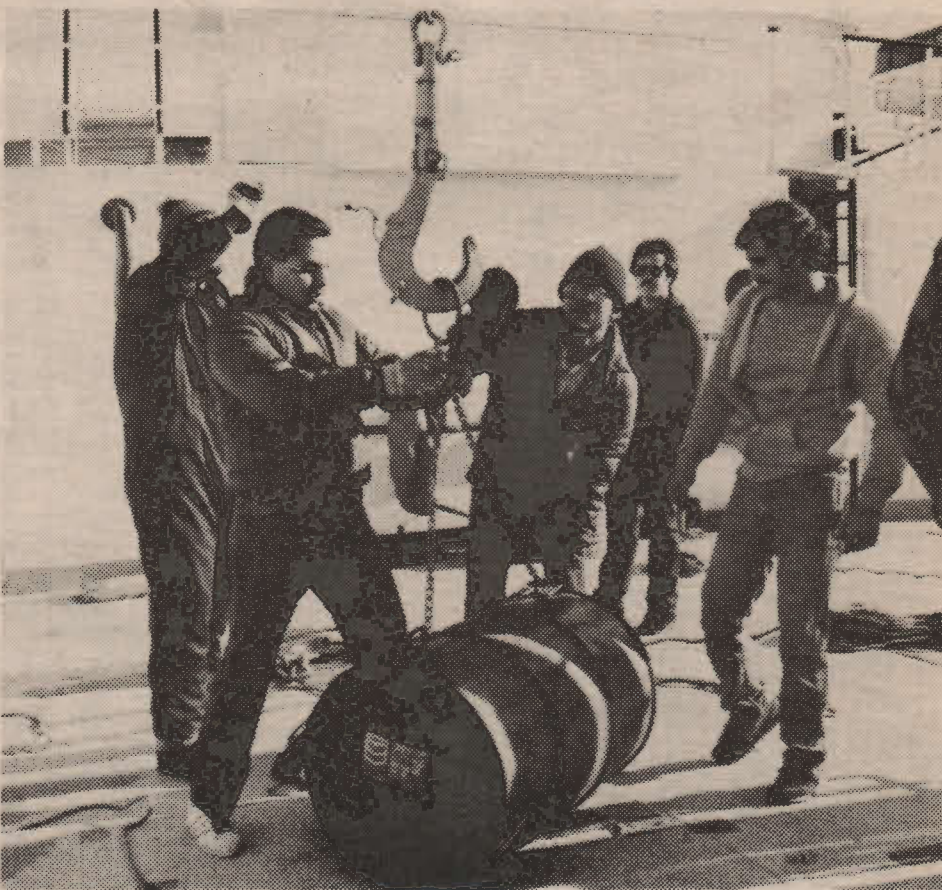
The chime hooks are disconnected after the drum is placed on deck.
