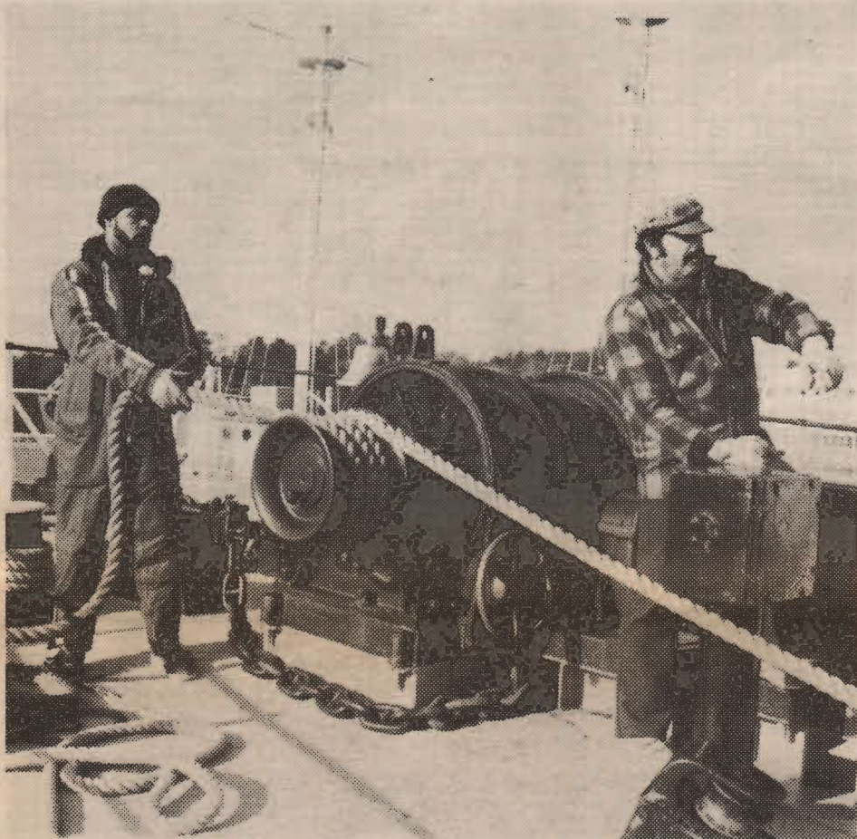
The highlines tension is checked by the ships windlass.
