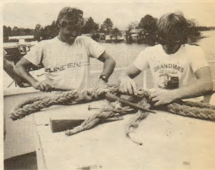
Rip Claunch (l.) and Curtis Dawson work on splicing an eight strand braid.
