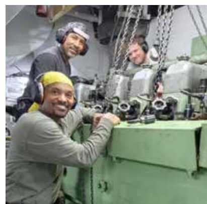
ABOARD CAPT. DAVID LYON – Generator head replacement takes place aboard the Sealift ship. Pictured from left are 1E John Nelson, 3E Lazaro Rivera Rodriguez, and OMI Nathan Bryant.
