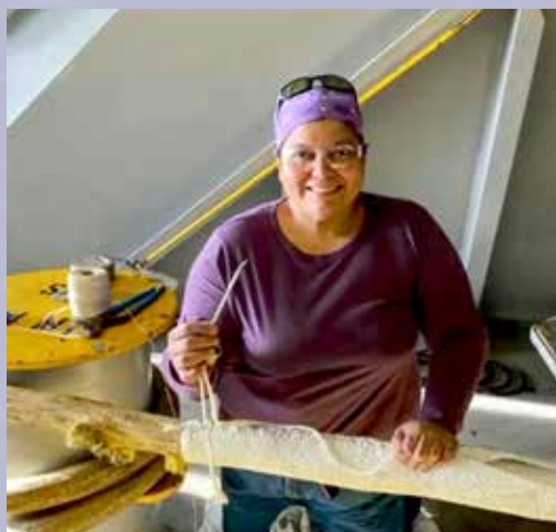
Colón Del Moral repairs the protective jacket on the mooring line.
